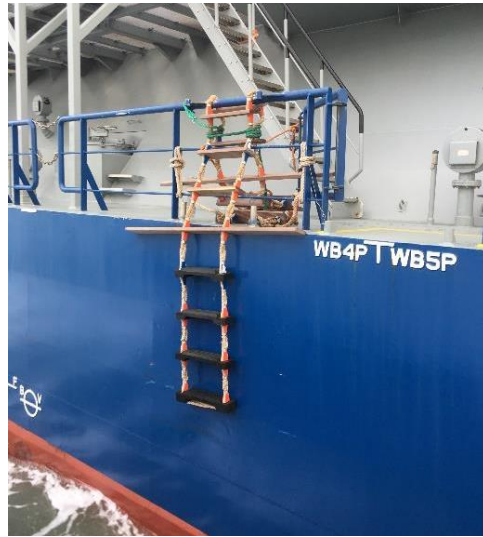
Example of a non-compliant Pilot Boarding Arrangement
